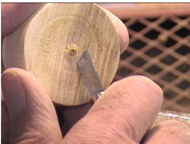
Carving tool to cut nib off bottom of box.
