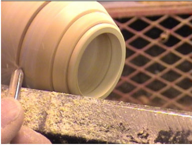
Detail gouge to finish shaping box.
