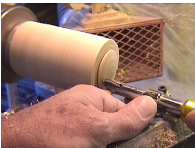
Detail tool to cut texture into lid.
