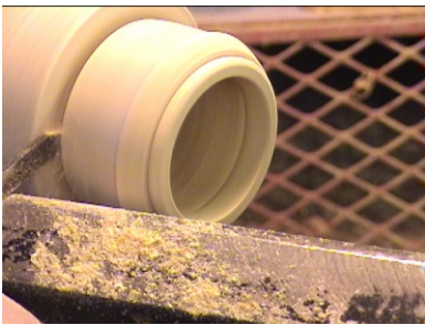
Parting tool to cut box off the blank.
